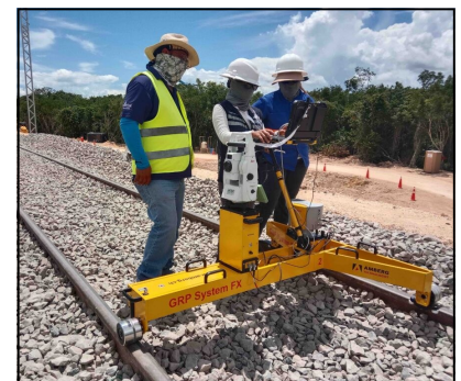
The Amberg IMS 1000 enabled a single team to do the work of three crews.
