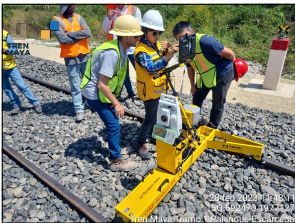
An Amberg survey team prepares for a rail inspection with their Amberg IMS1000.
